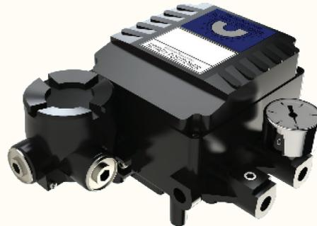
Most basic positioners have linear characterization. This means that the input signal to output rotation is directly proportional, which enables the process engineer to select a valve that will provide system characteristics. Standard ball valves, for example, provide equal percentage flow like many other quarter-turn valves do.
